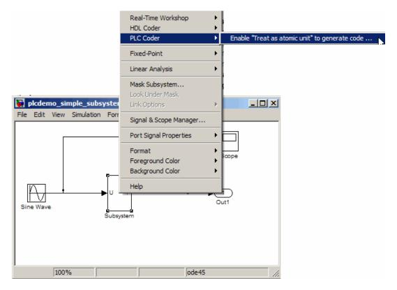
This command opens the block parameter dialog box so that you can select the **Treat as atomic unit** check box.
